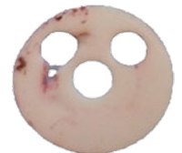
Worn Out Seal
